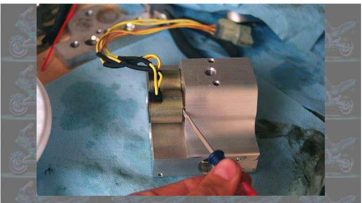
8) Remove the springs and spools behind the solenoid valves--pay close attention to the orientation of the spool as you remove it--you may have to turn the housing upside down and let them slide out. Once removed, look inside the spool and you'll see the tiny orifice. If this gets plugged, the system is hosed--that's why almost any gunk or particles cause such a mess.
