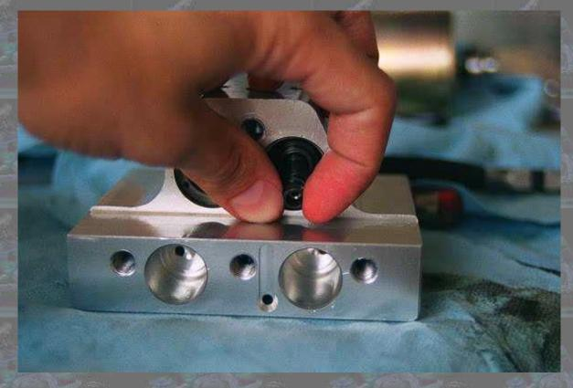
9) Disassemble the return pumps. Look at picture "disassembled return pump 1" below. These parts are a precision press-fit and need to be disassembled in a linear manner. I didn't take pictures (unfortunately) as I was taking them apart. If on a lathe, chuck one part in the headstock and use the drill bit chuck in the tailstock to hold
