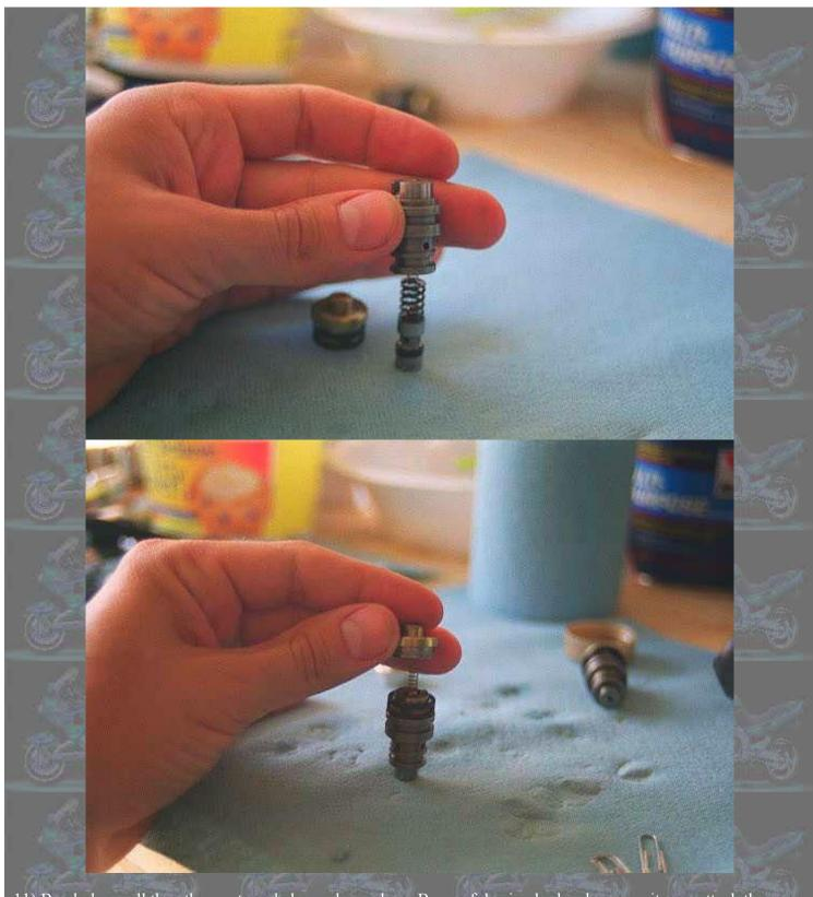
11) Break down all the other parts and clean, clean, clean. Be careful using brake cleaner as it may attack the o-rings--I used WD-40. Use the bronze (steel) wool to scrub off as much corrosion as you can from the steel parts. You may use naval jelly or a Dremel tool, whatever. Spray clean all of the passageways in the housing.
